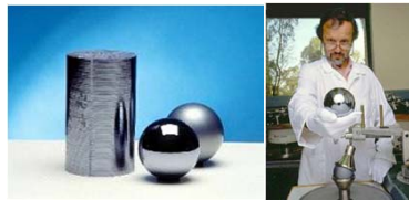
The standard ^{28}\text{Si} kilogram Spherical to 0.6 nm
